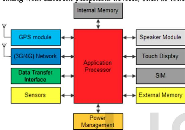
Fig. 2. General architecture of a modern smartphone. and video camera [34]. The ARM Cortex-A chips series introduced processors designed for smartphone applications. The Cortex-A15 MPCore processor is the latest of the Cortex-A series and it is based on ARMv7-A Cortex architecture with processor speed up to 2.5 GHz [35]. Exynos 5 Dual core is the Samsung Galaxy SIII AP, based on the ARM Cortex-A15 processor with clock speed up to 1.7 GHz [36].
