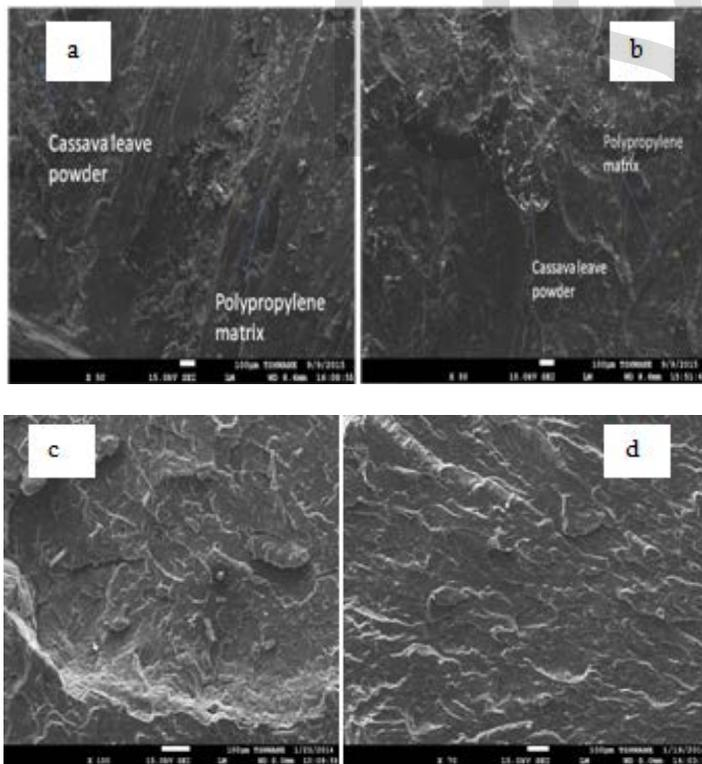
Fig.3. (a) Representative SEM photomicrograph of the composite having 3wt% cassava leaf powder particles dispersed in the polypropylene matrix; (b) Representative SEM photomicrograph of the composite having 5wt% cassava leaf powder particles dispersed in the polypropylene matrix.
