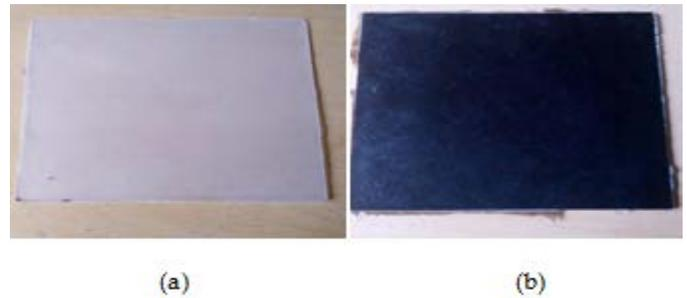
Fig.1. Extruded polypropylene based composites produced for (a) pure polypropylene, (b) Cassava leaf powder reinforced with polypropylene.
