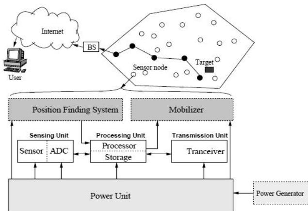
Figure II(b) : Components of a Sensor node
