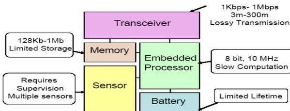
Figure II (a) : Layout of a node [3]
