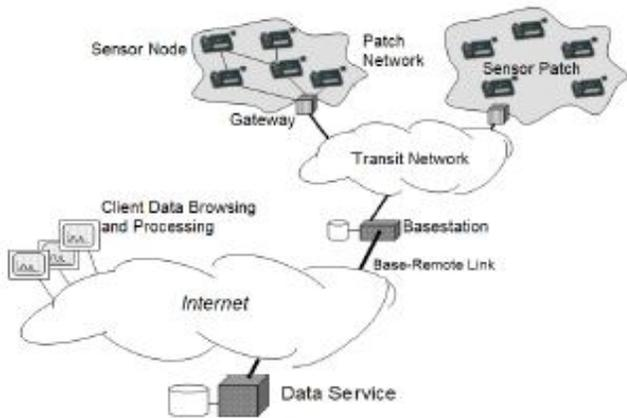
Fig. I: Layout of Wireless Sensor Networks [2]
