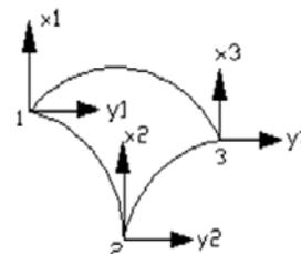
Fig. 3. Shallow Triangular Element
