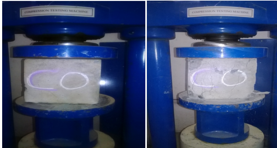
Fig1: cube kept in CTM before testing (left) cube kept in CTM after testing (right)
