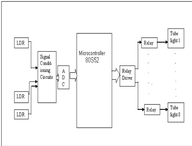
**Fig 1.2 Block diagram of developed lighting control system**
