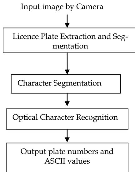
Fig 1: Flowchart of a Typical ALPR System
