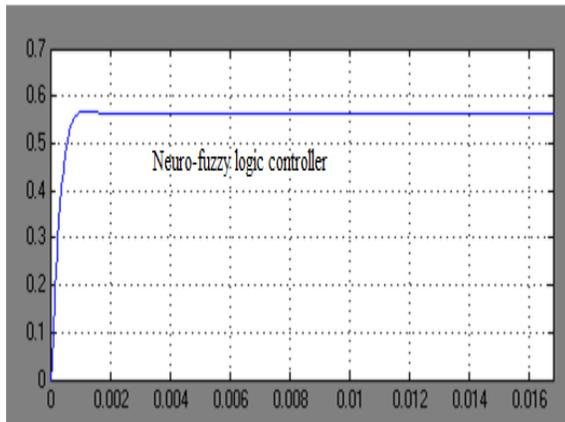
Figure 9 Step response of output (speed in p.u.) of the system BLSECD motor with Neuro-Fuzzy logic Controller
