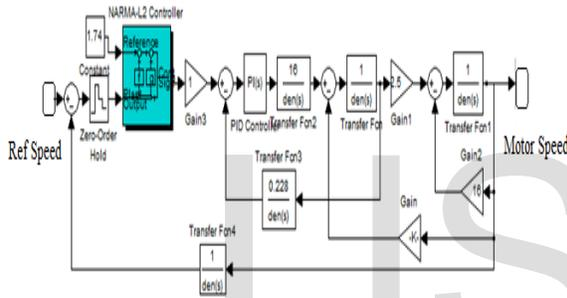
Figure: 6 Implementation of Neuro-Fuzzy logic controllers in SIMULINK for speed control of BLSEDC Motor
