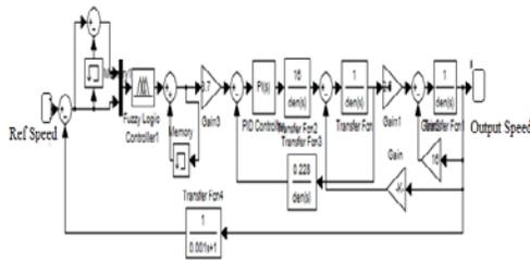
Figure 3 Simulation Model of the speed control loop for BLSEDC Motor using Fuzzy logic controller
