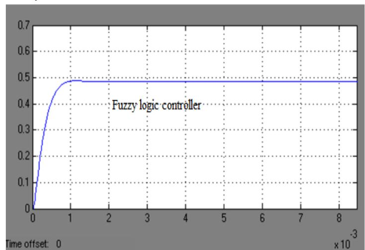
Figure 8 Step response of output (speed in p.u.) of the system BLSECD motor with Fuzzy logic Controller
