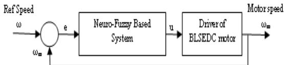
Figure: 5 Block Diagram of neuro-fuzzy logic controller of BLSEDC Motor for Speed Control
