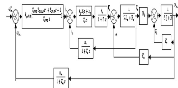
Figure 2: Simulation Model of the speed control loop for BLSEDC Motor using PID controller
