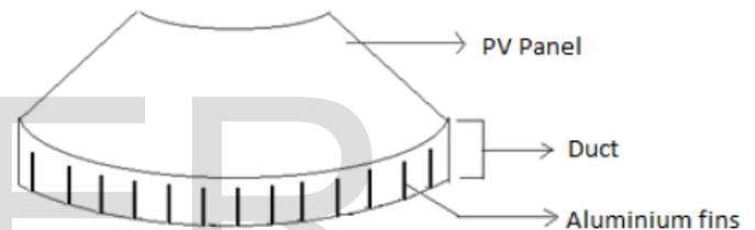
Fig 7: Part of the PV panel in the proposed model indicating the cooling system
