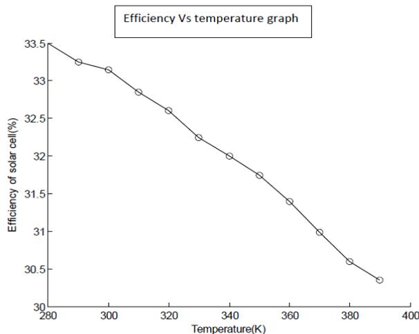
Fig 6: Efficiency of Solar panel at different temperature
