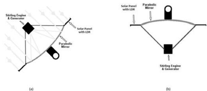
Fig 1: Design of the proposed solar model (a) Stirling engine during day (b) Stirling engine after sun set
