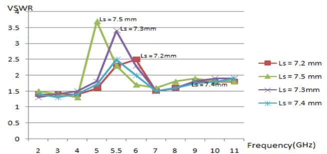
Fig. 4: variation of the simulated VSWR with different slot length ( $L_s$ ) in the ground plane.
