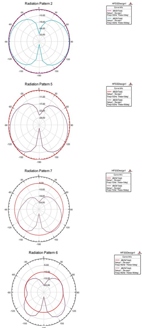
Fig. 8. Simulated radiation far-field patterns for the proposed antenna operation at (a) 3 GHz, (b) 5 GHz, and (c) 7 GHz and (d) 9GHz
