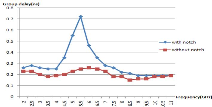
Fig. 7: simulated group delay of antenna with and without notched.
