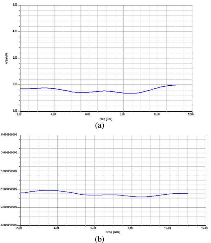
Fig. 2 Simulated VSWR and Group delay of antenna (a) without notch with optimal dimensions.
