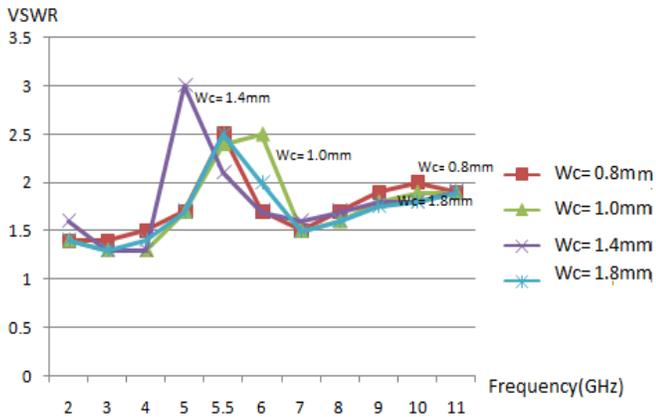
Fig. 6: variation of the simulated VSWR with different location of the slot ( $W_c$ ) in the ground plane.
