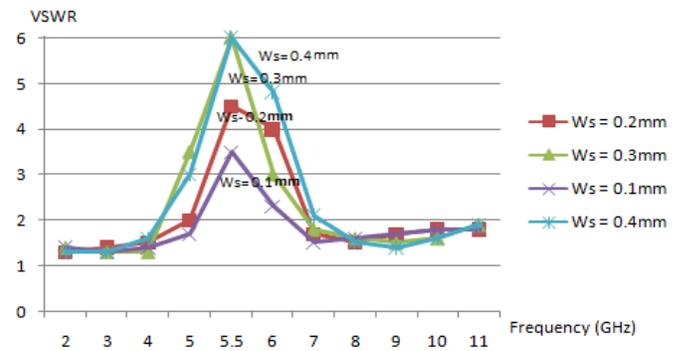
Fig. 5: variation of the simulated VSWR with different slot widths ( $W_s$ ) in the ground plane.
