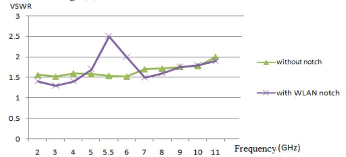
Fig. 3: Simulated VSWR of antenna with WLAN notch and without notch
