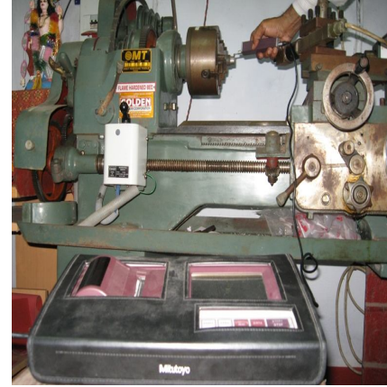
Fig.3. Surface Roughness Surf test – SJ-301
