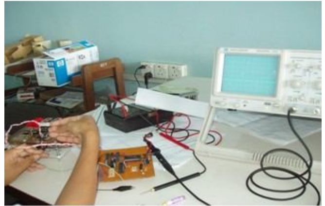
Fig. 15. Testing the received voltage level at the display unit.
