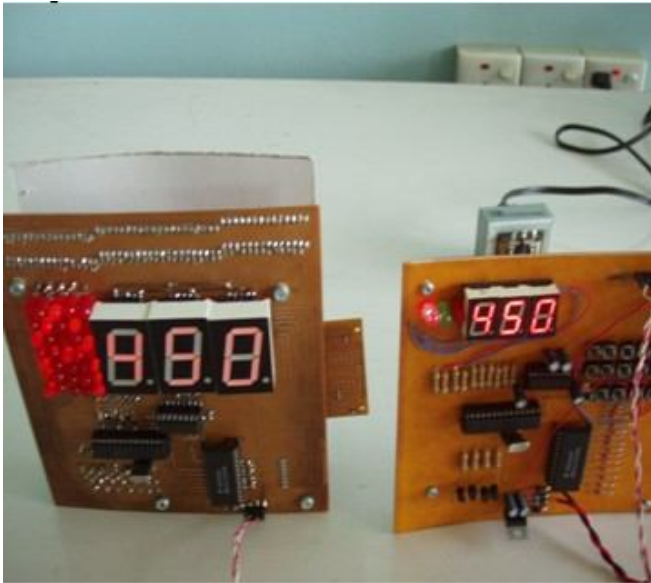
Fig. 13. Testing the receiving data both console unit and display unit in remote display system.
