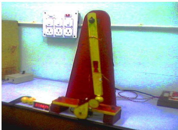
Fig 5 Experimental setup for impact fatigue testing
