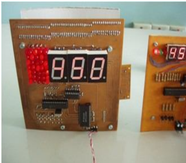
Fig. 14. The display unit with the data receiving process.
