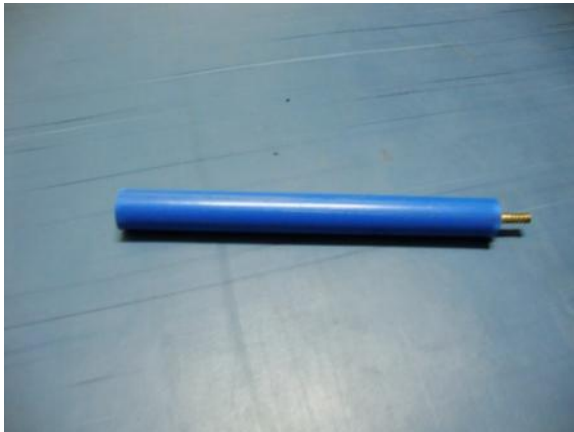
Fig 5.4.3: Pespex pipe of 2inch diameter and 12 inches length with 1 inch aperture with 3/4 th inch brass gas inlet nozzle.
