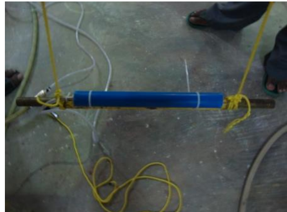
Fig 5.4.4: Pespex pipe assembly connected to 3/4 th inch air hose with rope and mounting arrangement with dead weight.
