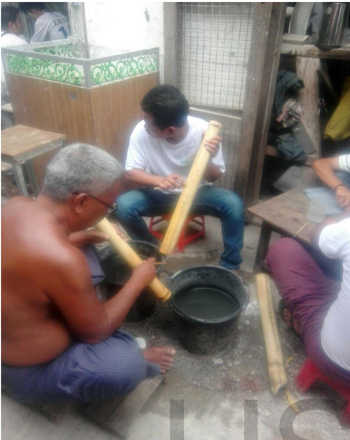
Further polishing of jade by bamboo
