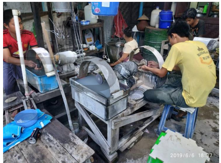
Jade cutting process with medium-sized machine
