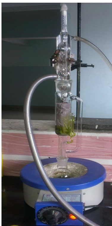
Fig 4.1 Soxhlet apparatus used for extraction of methanolic extracts of the selected plants
