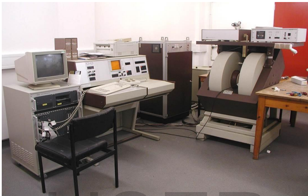
Figure 3.1: Picture showing Bruker ESR system.
