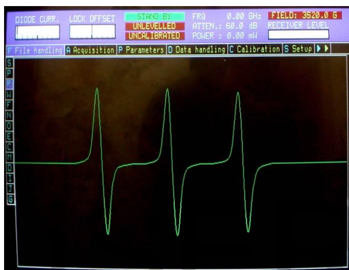
Figure 3.6: Typical spectrum observed in the Bruker ESR system.
