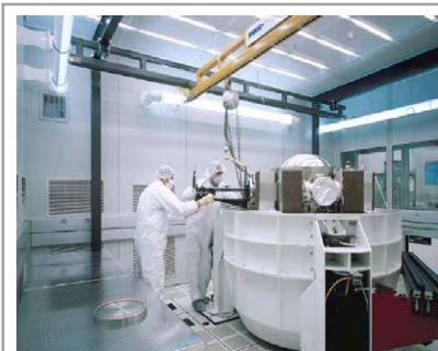
Figure 3.45: NIST's experimental Molecular Measuring Machine for ultraprecise two dimensional measurements in one of the AML's underground metrology wings. The instrument is designed to be operated by remote control from the adjoining room to minimize environmental disturbances. The instrument is used to draw lines on silicon as small as 10 nanometers wide and 4 nanometers high. It can also measure the placement of nanometer-scale features with subnanometer resolution. [Source is http://www.google.com/eg/search Nanotechnolog world, Retrieved 20 November, 2011]
