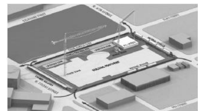
Figure 2.116: 3D Architectural Model and Site Logistic Planning Model
