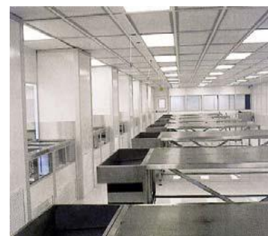
Figure 3.49: Cleanroom furniture is designed to produce a minimum of particles and to be easy to clean. [Source is http://www.google.com/eg/search Nanotechnolog world, Retrieved 20 November, 2011]
