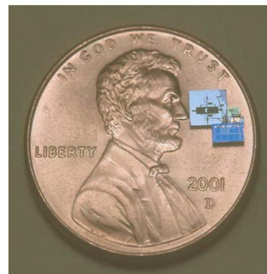
Figure 3.30: Smart dust. The visions for smart dust presume that it will be relatively undetectable by the human eye. Current research efforts have dramatically brought down the size of the dust. (Berkeley)
