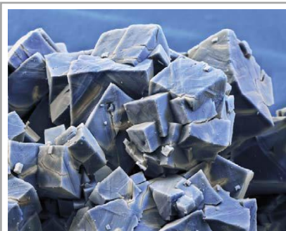
Figure 3.10: Developing a way to store energy-rich gases can help our energy systems. Metal organic frameworks (MOFs) are highly porous organic matrix substances that can store hydrogen or natural gas. The cubical nanostructures consist of an “organometallic” framework, whereas the interior of the cube contains numerous nanometersize pores in an interconnected structure. The nanopores have high surface area. These structures might also be used for energy sources for many devices, such as laptops. Tiny fuel cells could serve as a rechargeable storage medium. (Courtesy of BASF.)
