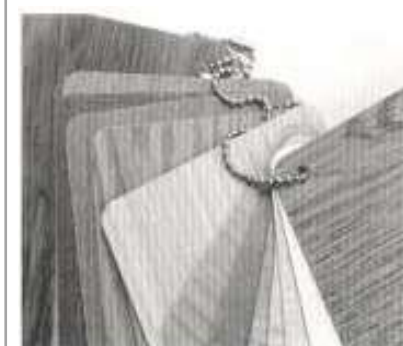
Figure 2.24: "Fakes" – laminates that simulate real materials. Real wood exhibits other haptic, acoustic and sensory properties than wood imitations.
