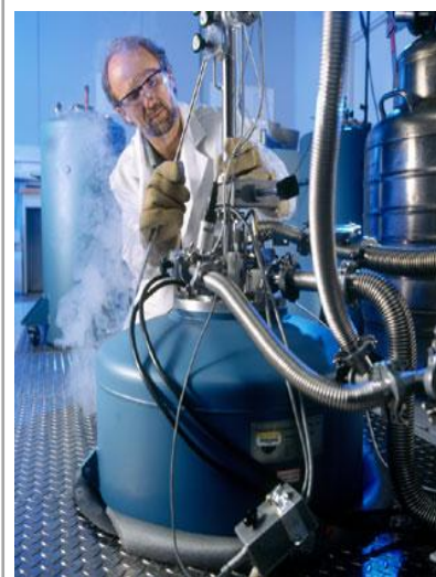
Figure 3.46: Ultraprecise electrical measurements require extremely stable temperature, humidity, and vibration control. Here, a NIST physicist in one of the AML's metrology laboratories prepares to measure the international standard for resistance— the quantum Hall Effect [Source is http://www.help-stop-globalwarming.com/global-warming-recycling.html , Retrieved 20 November, 2011]
