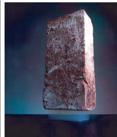
Figure 2.93: Aerogel has a density only three times that of air, but it can support significant weights and is a superb insulator. Aerogels were discovered in 1931 but were not explored until the 1970s. (NASA)
