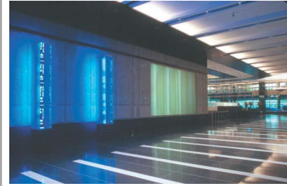
Figure 2.126: Fiber-optics, dichroic glasses and LEDs were used by James Carpenter Design Associates in this lobby installation for Bear Stearns in New York. The green zone is produced with fiber-optics and dichroic glass, it serves as a soft contrast to the moving blue LED information screens.
