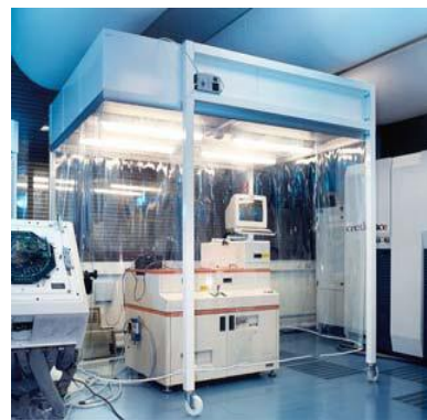
Figure 3.47: Clean room cabin for Precision measuring tools. [Source is http://www.google.com/eg/search Nanotechnolog world, Retrieved 20 November, 2011]
