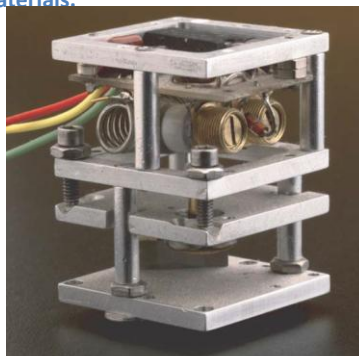
Figure 3.27: This microseisometer is capable of sensing accelerations. Thus, it can be used for sensing vibrations. (NASA)
