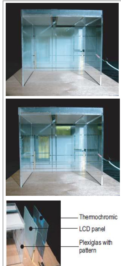
Figure 2.124: Design experiment: the patterns in this wall study vary with changing temperature and with the on-off state of the LCD panel. (Yun Hsueh)
