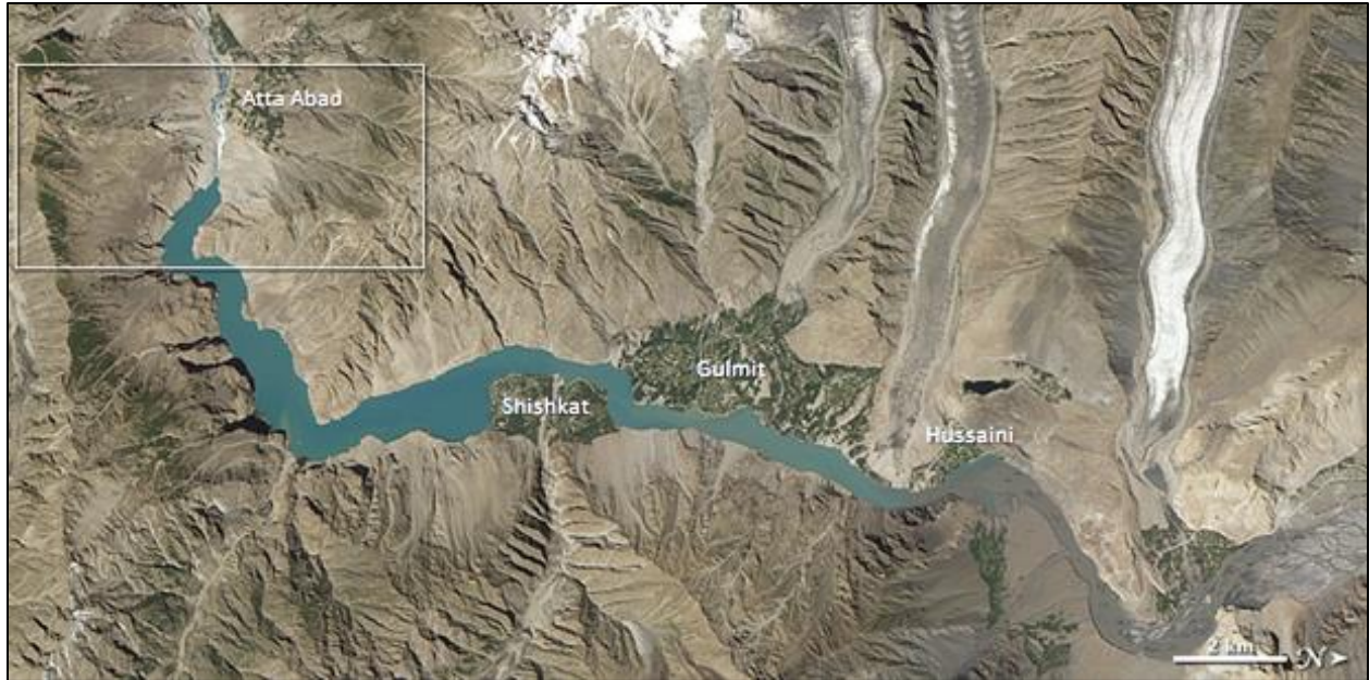
Figure 2.15: Lake (blue-green) lingering behind the earthen dam in this true color image, acquired on Aug.3, 2011 by ALI on NASA's Terra satellite. Dam crest changed slightly between July 2010 and August 2011, also spillway revealed into the box area. North arrow is at right due to rotation of image.
