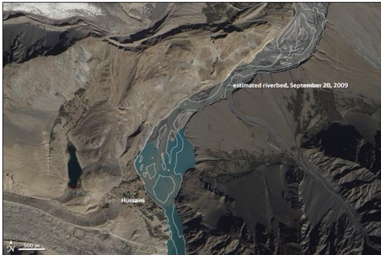
Figure: 2.14: NASA's EO-1 satellite acquired this natural color image on Oct.3, 2010 by ALI, suggesting the decline in water level at upstream margin of lake since July, 2010 and river also returning to its former bed whereas long shadow describing the change in season in this scene
