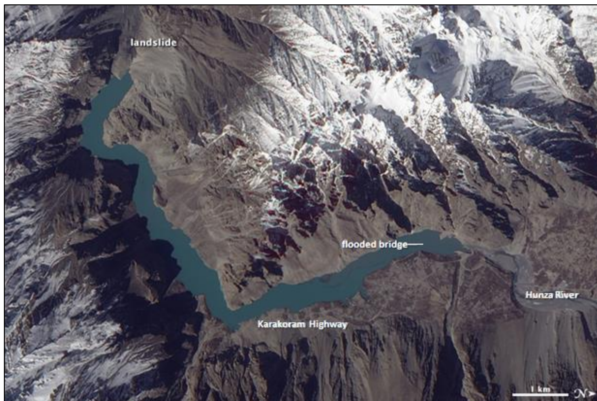
Figure 2.5: EO-1 satellite image acquired from http://earthobservatory.nasa.gov/ on March 16th 2010 displaying the Attabad landslide in Northwest Pakistan and debris dam and the extent of landslide-dammed Lake Attabad, 72 days after impoundment. The image has been rotated so that north is to the right.
