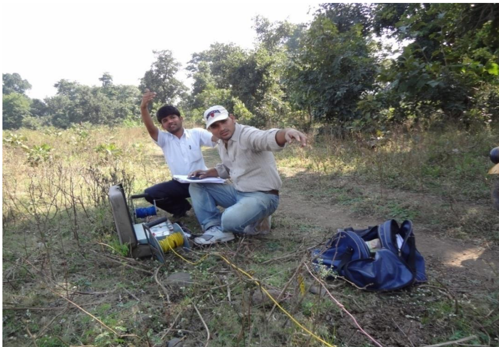
PHOTO 5.2: Vertical electrical Sounding at Somarpet village.
