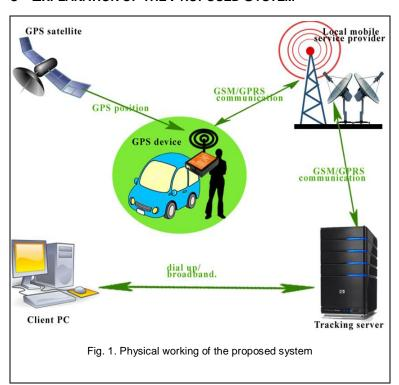
The Physical Components of Tracking System are
