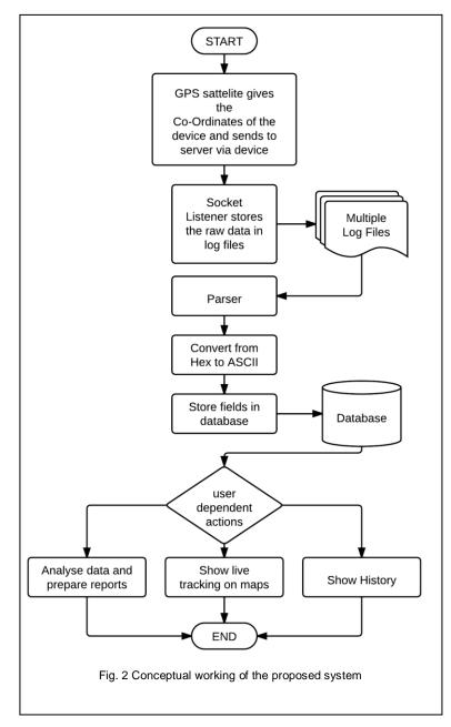
As we have seen in the previous section GPS Satellite gives the position of the AVL device in the form of latitude, longitude and altitude. All this information is then given to the Server which is received by the socket listener onto a particular port of the server. The data which is received is in the hex format which is non readable to humans.
