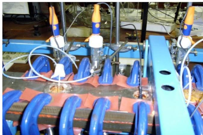
Figure 7A: Rig with the sensor probe for pH measurements
