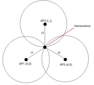
Figure 2. Trilateration algorithm.
