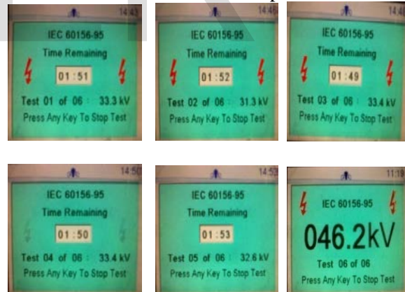
Figure 13: Laboratory Test Results of Silicon, Paraffin and Naphtha oil break down voltage at 30°C
