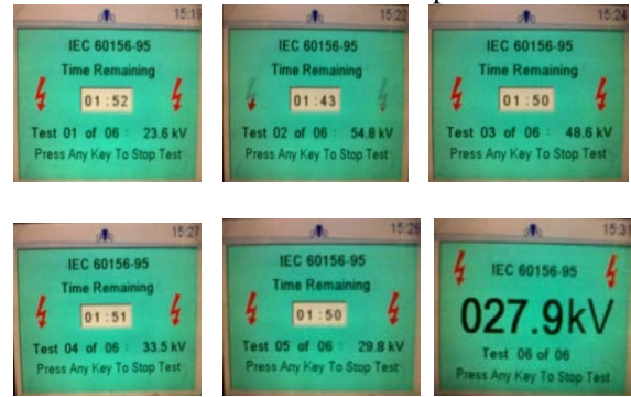
Figure 16: Laboratory Test Result of Silicon, Paraffin and Naphtha oil break down voltage at 60°C
