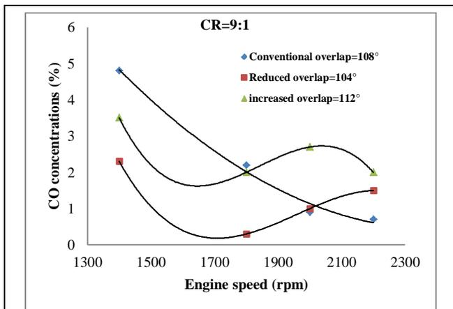
Fig. 9. The impact of VVT on CO for variable engine speeds at CR=9:1.
