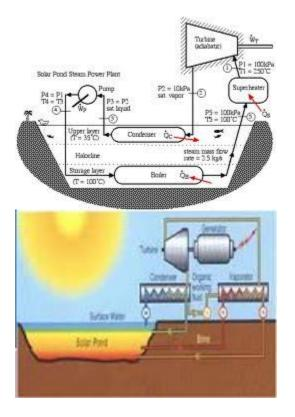
A solar pond is a pool of saltwater which acts as a large-scale solar thermal energy collector with integral heat storage for supplying thermal energy. A solar pond can be used for various applications, such as process heating, desalination, refrigeration, drying and solar power generation.
