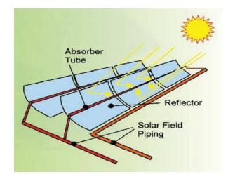
Parabolic trough power plants use concentrated sunlight, in place of fossil fuels, to provide the
