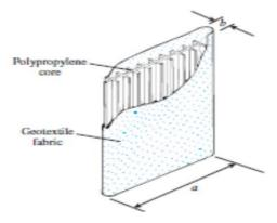
Fig. 3. Prefabricated Vertical Drains (after, Das 1983)
