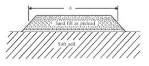
Fig. 1. Soil improvement by preloading (after, P.C.Varghese 2005)
