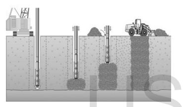
Fig. 4. Installation process of stone column (after, Hussein 2006)
