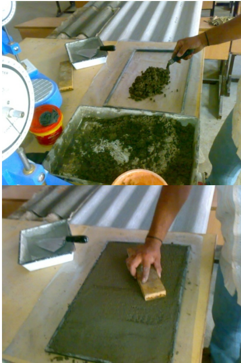
Fig 24. Spreading and Smoothing with hand trowel
