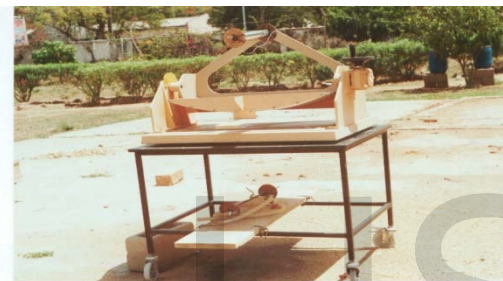
Fig. 6. Basic Components of the Parabolic-Trough Collector
