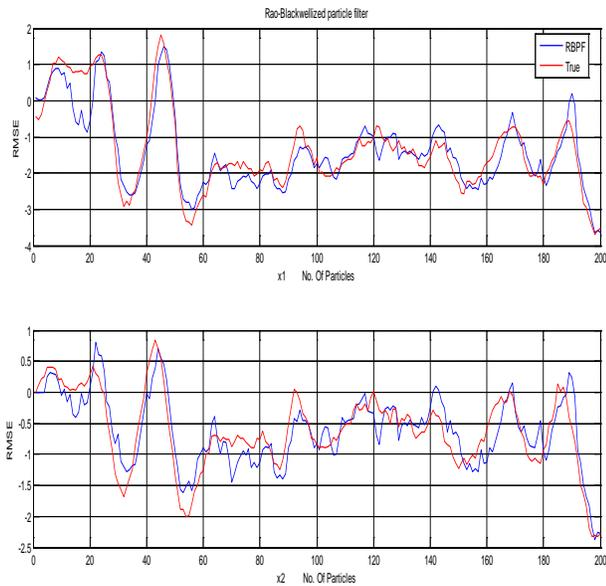
**FIG-2: RMSE Estimation of Rao-Blackwellised Particle Filter using 10 Monte Carlo simulation with N = 200 particles.**
