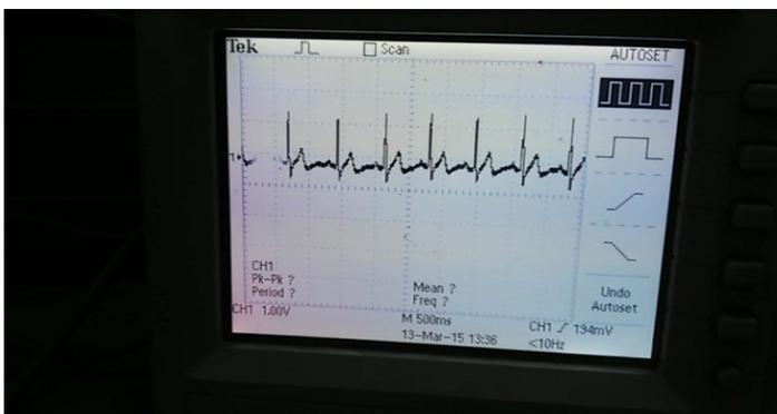
Fig.4: ECG signal observed on the oscilloscope
