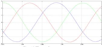
Fig. 13 Three phase stator current
