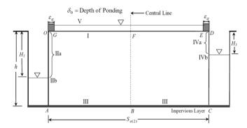
**Fig. 2.** Geometry of a fully penetrating ditch drainage system with unequal water level heights in between adjacent drains and subjected to a uniform depth of ponding at the surface of the soil
