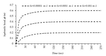
**Fig. 6.** Graph showing the comparisons transient hydraulic head variations for problem Fig. 1 wr.t different Specific storages (Ss) for flow following situations  $\varepsilon_a = 0.1$ m and the other soil parameters are taken as  $K_x = 0.05$  m/day;  $K_y = 0.05$  m/day;  $H_1 = H_3 = 0.5$  m.
