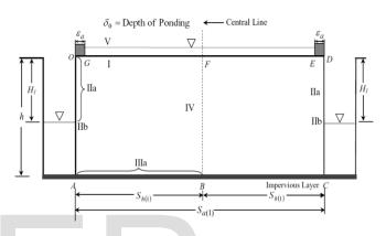
**Fig. 1.** Geometry of a fully penetrating ditch drainage system with equal water level heights in between adjacent drains and subjected to a uniform depth of ponding at the surface of the soil.
