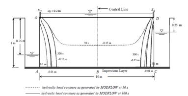
**Fig. 4.** MODFLOW generated contours for the proposed flow problem of Fig. 2 for a flow situation at corresponding time intervals (50 s and 300 s), when  $\varepsilon_a = 0.1 \text{ m}$  and the soil parameters are taken as  $S_s = 0.001 \text{ m}^{-1}$ ,  $K_x/K_y = 1/1$  ( $K_x = 0.5 \text{ m/day}$ ,  $K_y = 0.5 \text{ m/day}$ ) when  $H_1 = 0.75 \text{ m}$  and  $H_3 = 0.25 \text{ m}$
