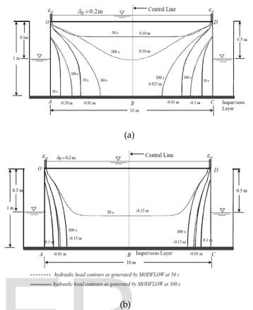
**Fig. 3.** MODFLOW generated contours of hydraulic head for the proposed flow problem of Fig. 1 for a flow situation at corresponding few time intervals (50 s & 300 s) when  $\varepsilon_a = 0.1 \text{ m}$  and the soil parameters are taken as  $S_s = 0.001 \text{ m}^{-1}$ and (a)  $K_x/K_y = 10/1$  ( $K_x = 0.5 \text{ m/day}$ ,  $K_y = 0.05 \text{ m/day}$ ) and (b)  $K_x/K_y = 1/1$  ( $K_x = 0.5 \text{ m/day}$ ,  $K_y = 0.5 \text{ m/day}$ )
