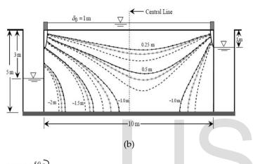
Steady-state hydraulic head contours as obtained vide Kirkham's solution (Fig. 2 & 3, 1965)
