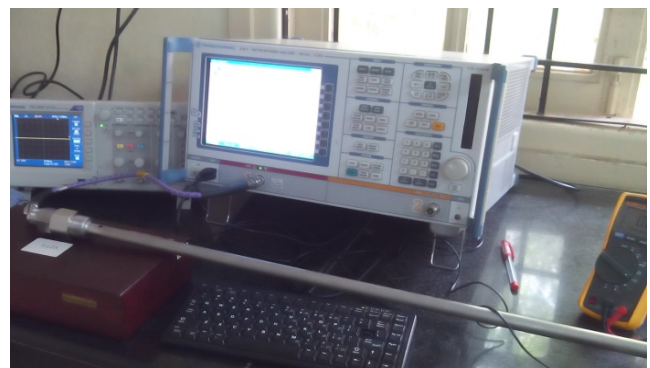
Fig 1. 2m Stainless steel waveguide testing with characteristic impedance of 50 \Omega .
