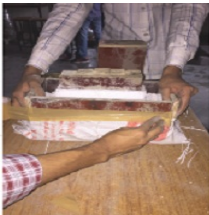
Fig. 3. Placing Gunny Bag as a base of the mould
