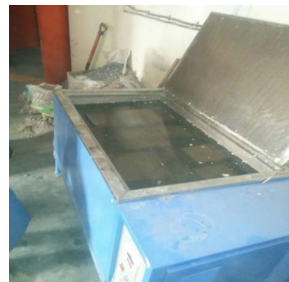
Fig. 5. Cubes in curing tank
