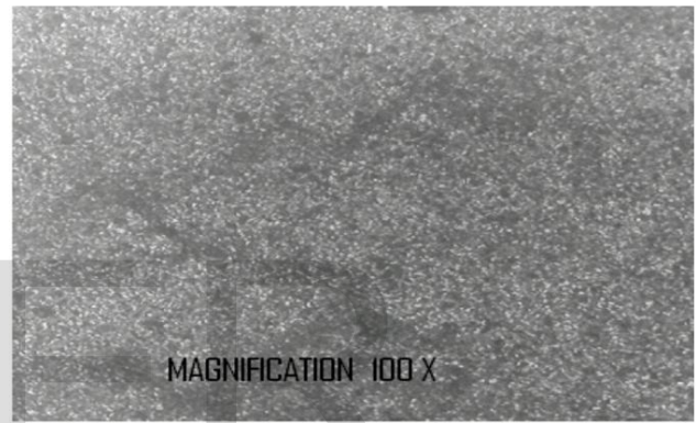
Fig. 5. Microstructure of cryogenic processed specimen
