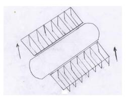
When the wings move up, they open automatically and the drag is minimized to zero, that time the drag is approximately equals to zero
