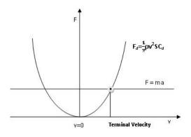
As we can see on the graphic, if we apply acceleration to our object, there will be a time when the force resultant to our acceleration equals to the drag force, at this time, the object will not accelerate anymore but it will have a uniform motion. After this point, the drag will be much bigger than the force we are applying to the object itself.
