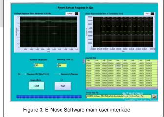
This VI also records the voltages from sensor modules during air environment around the sensor array, which are the voltages across load resistance RL.The user has to choice to choose number of samples and sampling time in seconds. After pressing SAVE button the acquired data shows in the waveform graph as time Vs sensor response acquired voltages. This VI automatically converts the voltage response into change in conductance of sensor (G) using below formulas. (1, 2, 3)
