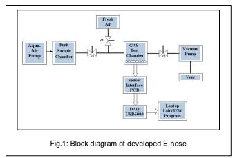
Figure. 1 shows a block diagram of fabricated E-Nose system, comprising a sensor array of eight sensors, gas test -chamber, fruit sample chamber, an interface printed circuit board (PCB), and DAQ card and user interface software for data acquisition, pre-processing, storage and classification as well as verification program
