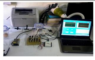
Fig.2 Fabricated E-Nose system
