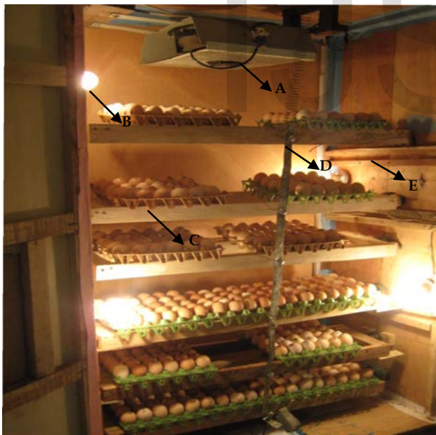
Fig. 5. The incubator loaded with eggs (A- Fan, B- 60 Watt electric bulb, C- egg tray rack, D- tray turning spring, E- thermocouple)
