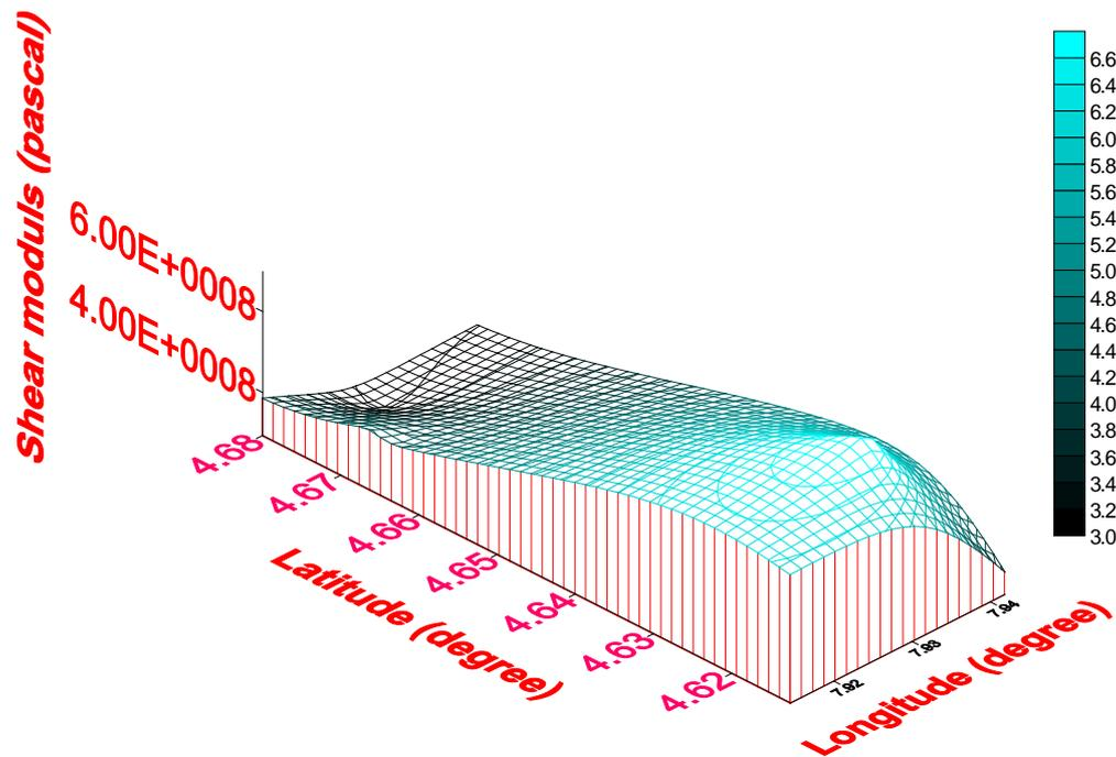
Figure 3: 3-D contour map of layer two first lame's constant (Shear modulus,  $\mu$ ) in the study area
