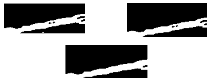
Fig. 7. (a) Binary image (b) Removal of smaller pixels (c) Removal of holes
