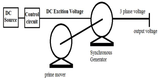
Fig. 5 Generator based VSG
