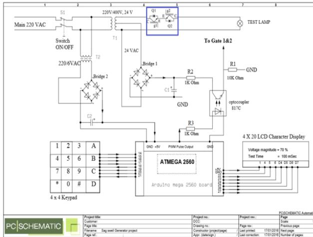
Fig.13 Schematic Diagram of VSSG
