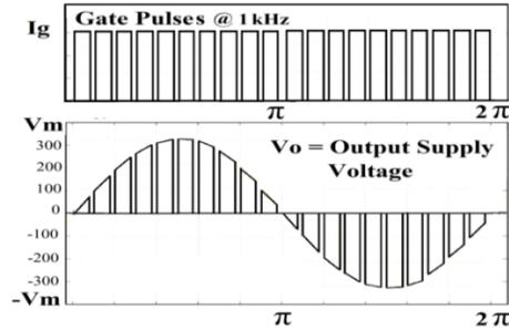
Fig .11 Multiple PWM pulses with 75% duty cycle and the output of AC Chopper
