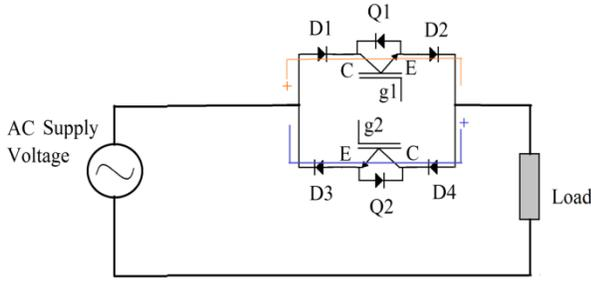
Fig.9 Switches are connected in anti parallel
