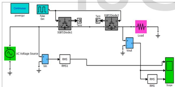
Fig.19 AC chopper with anti-parallel connected IGBTs in MATLAB Simulink
