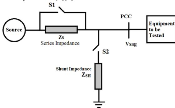
Fig. 1 Impedance switching VSG
