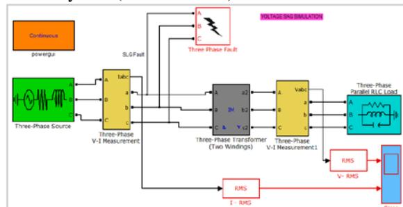
Fig.17 MATLAB Simulation of voltage sag due to SLG fault
