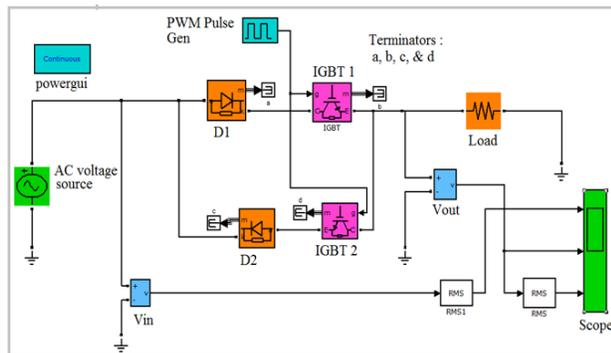
Fig.20 AC chopper with anti-parallel connected IGBTs in MATLAB simulink
