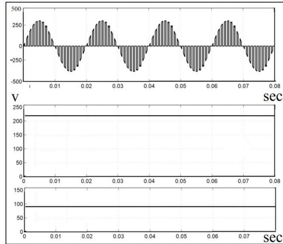
Fig.21 Output chopped wave form at 50% duty cycle for anti parallel and series connected IGBTs.
