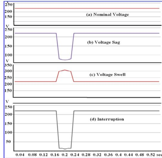
Fig.16 Output RMS voltage of sag and swell generator (a) Nominal voltage (b) voltage sag (c) voltage swell (d) voltage interruption
