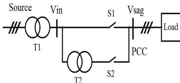
Fig. 7 AC Chopper based VSG
