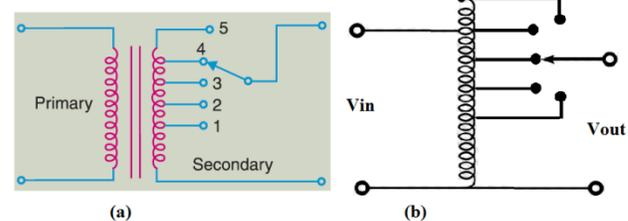
Fig. 3 (a) Multiple tap transformer
