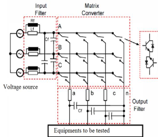
Fig.6 Matrix converter based VSG
