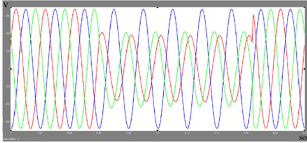
Fig.18 Transformer secondary voltage wave form due to SLG fault on primary side for duration of 10 cycles (50Hz) or 0.2sec (for Δ/Y ungrounded connection)
