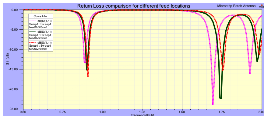
Figure 3: Return loss with change in Feed location
