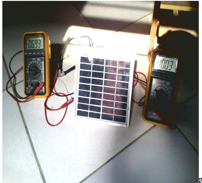
Figure 5.1 (a) Setup of the PVL-1241 solar laminate panel in Summer at temperature 39°C.
