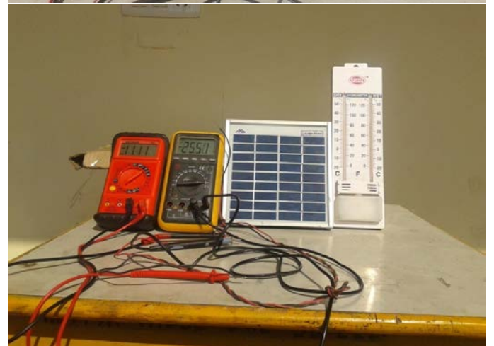
Figure 5.1 (b) Setup of the PVL-1241 solar laminate panel in winter at temperature 15°C
