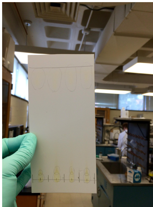
Fig. 2 The plastic-backed TLC plate used in the experiment – the areas of alliin concentration have been circled in pencil. Going in order from bottom to top, the lowest and low concentrations of alliin are at the bottom and the high concentration is at the top.
