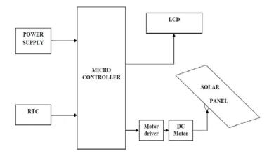
Fig.3: Block diagram of the Time operated solar tracking system using RTC
