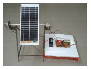
Fig 4: Prototype of Time operated solar tracking system using RTC
