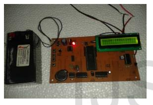
Fig 5: Control equipment of solar tracking system
