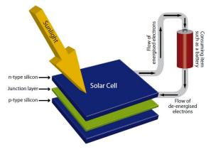
Fig.1:Principle of operation of a PV Cell.
