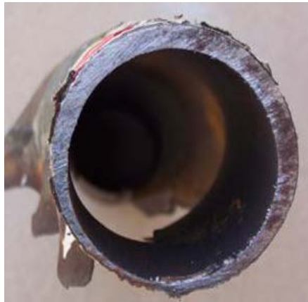
Figure 11. Photograph of the cross-section of the showing thinning of the tube
