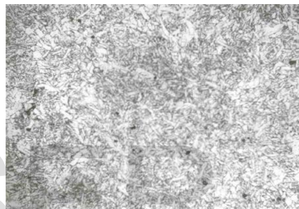
Figure 6. Photomicrograph of a cross-section of economizer tube at the weld 200 X
