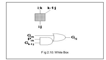
The kogge stone adder the generate and propagate blocks produce the caay and sum such that each block output will act as input to the next block and in the same way such that the final sum is being produced . the below figure represents the schematic how the generation and propogation of carry is done for the production of the final sum
