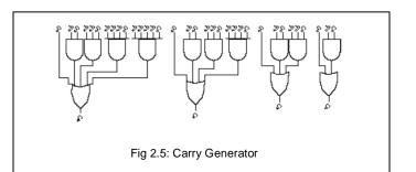
The size and fan-in of the gates needed to implement the Carry-Look-ahead adder is usually limited to four, so 4-bit Carry-Look ahead adder is designed as a block. The 4-bit Carry Look Ahead adder block diagram is shown below
