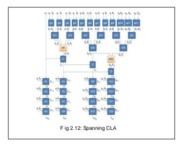
In this spanning CLA a reduction of number of stages is being done by reduceing the genration and propagate units . the ouputs of the previous GP units are being considered such that the combination of consecutive Gp units produces carry once and that one is being given as inout to the next stage .
