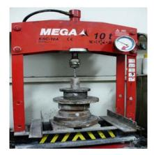
Fig.2. MEGA.KSC-10 hydraulic press
