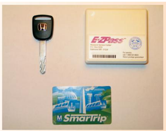
Fig. 5 Some car keys (upper left) contain a passive tag. An EzPass (upper right) helps collect highway tolls, a Smart Trip card (bottom) collects fares in a public transit system.
