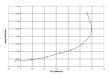
**Fig. 5.5.** Lift to Drag Ratio Curve of Aerofoil Shaped Fuselage Model at 20 m/sec
