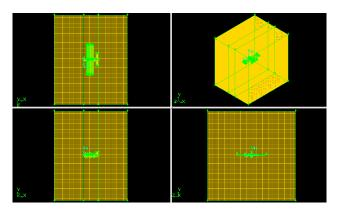
**Fig. 2.2** Different Views of CylindricalShaped Fuselage Model after Meshing.
