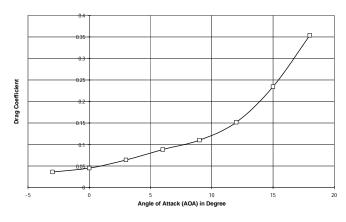
**Fig. 4.6.** Variation of Drag Coefficient with Angle of Attack for Aerofoil Shaped Fuselage Model at 20 m/sec.
