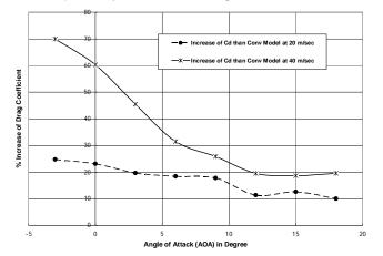
**Fig. 5.10:** Percentage Increase of Drag Coefficient of "Aerofoil shaped fuselage configuration at 40 m/sec" than that of "Cy-lindrical shaped fuselage configuration at 20 m/sec & 40 m/sec" respectively and Different Angle of Attack.
