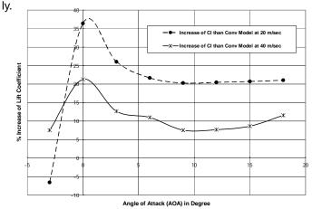
**Fig. 5.7** Percentage Increase of Lift Coefficient of "Aerofoil shaped fuselage configuration at 20 m/sec" than that of "Cy-lindrical shaped fuselage configuration at 20 m/sec & 40 m/sec" respectively and Different Angle of Attack.
