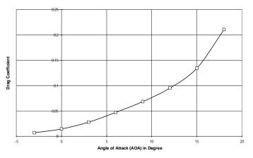
**Fig. 4.4.** Variation of Drag Coefficient with Angle of Attack for Cylindrical Shaped Fuselage Model at 40 m/sec.
