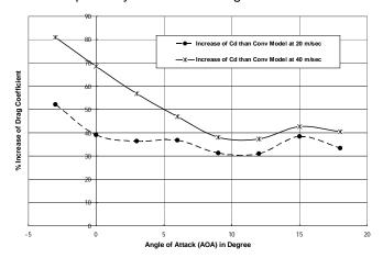
**Fig. 5.8** Percentage Increase of Drag Coefficient of "Aerofoil shaped fuselage configuration at 20 m/sec" than that of "Cy-lindrical shaped fuselage configuration at 20 m/sec & 40 m/sec" respectively and Different Angle of Attack.
