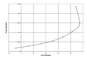
**Fig. 5.3.** Lift to Drag Ratio Curve of Cylindrical Shaped Fuselage Model at 20 m/sec
