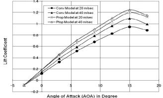
Fig. 5.1. Comparison of Lift Coefficient with AOA of Different Models.
