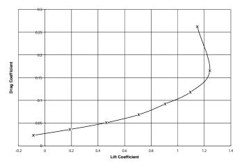
Fig. 5.6. Lift to Drag Ratio Curve of Aerofoil Shaped Fuselage Model at 40 m/sec
