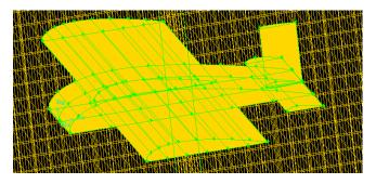
Fig. 2.4 Aerofoil Shaped Fuselage Model after Meshing.
