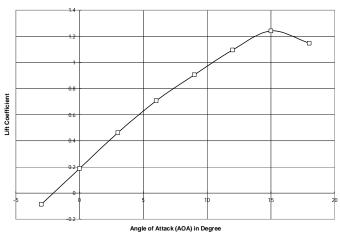
**Fig. 4.7.** Variation of Lift Coefficient with Angle of Attack for Aerofoil Shaped Fuselage Model at 40 m/sec.
