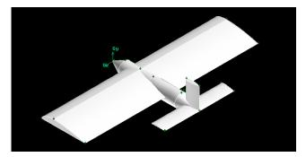
Fig. 3.1. Isometric View of Cylindrical Shaped Fuselage UAV Model.
