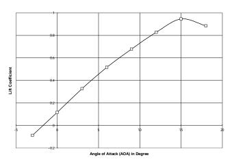
**Fig. 4.1.** Variation of Lift Coefficient with Angle of Attack for Cylindrical Shaped Fuselage Model at 20 m/sec.
