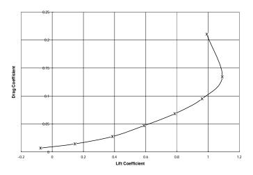
**Fig. 5.4.** Lift to Drag Ratio Curve of Cylindrical Shaped Fuselage Model at 40 m/sec
