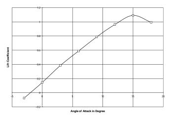
**Fig. 4.3.** Variation of Lift Coefficient with Angle of Attack for Cylindrical Shaped Fuselage Model at 40 m/sec.
