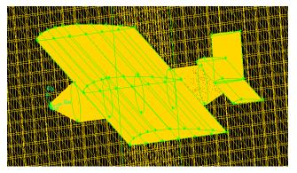
Fig. 2.1 Cylindrical Shaped Fuselage Model after Meshing.
