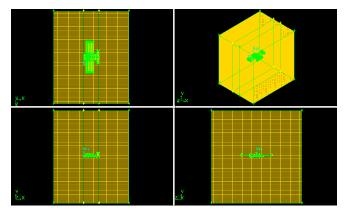
**Fig. 2.5** Different Views of Aerofoil Shaped Fuselage Model after Meshing.
