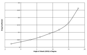
**Fig. 4.8.** Variation of Drag Coefficient with Angle of Attack for Aerofoil Shaped Fuselage Model at 40 m/sec.
